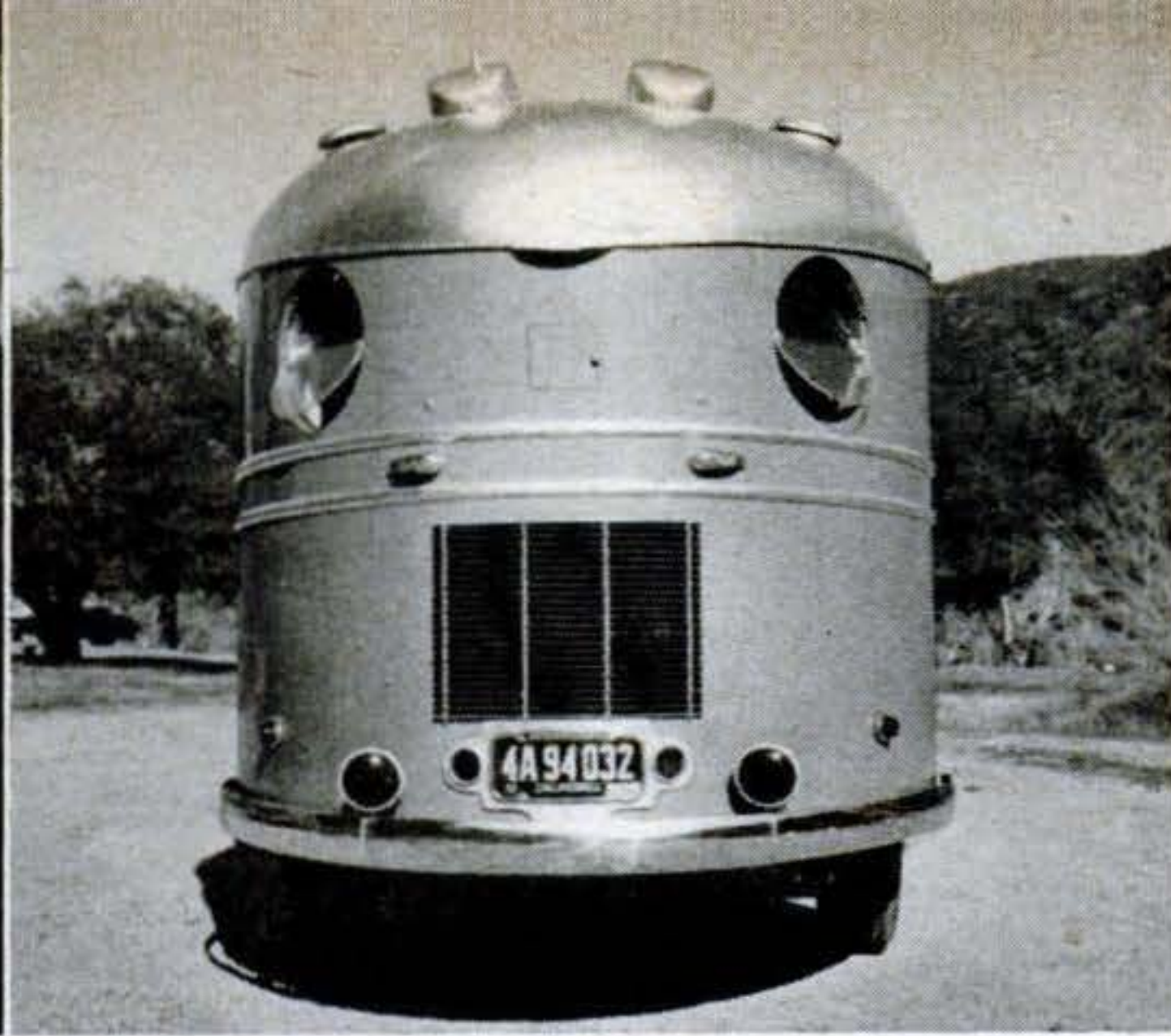
ROUND PLASTIC WINDOWS in rear help ventilate cabin. Ford bus radiator is in center. Side louvers force air through engine compartment while coach cruises, often at 60 m.p.h.
